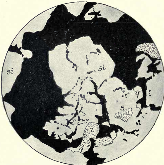
Replaced Quartzite, Same Locality as Fig. 16. Black, galena; z , zinc-blende; q , quartz; s , sericite; si , granular siderite. Quartzite in same section gradually changing to this ore. Magnified 35 diameters.
